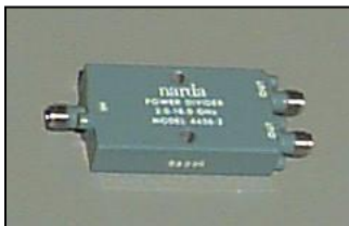
Figure 2 – Narda power divider in the 2 to 18 GHz range
