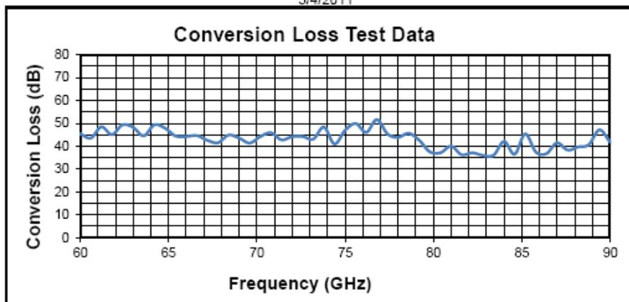
Optimized for Agilent PSA: R.F. = -30 dBm, L.O. = (RF+IF)/16 @ 15.5 dBm, I.F. = 321.4 MHz, Bias = 6.78 mA
