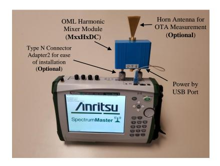
OML has developed a frequency extender module solution that can be used with Anritsu's SpectrumMaster. With this harmonic mixer making millimeter wave measurements in the field are now at your fingertips.
