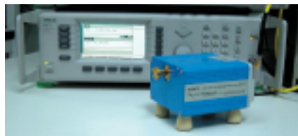
▲ Fig. 1 The OML Source Module being used to extend the frequency range of a lower frequency signal generator.
